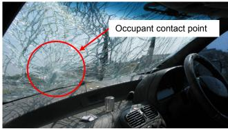
Figure 3B: Roof crush measured is 18 cm and occupant contact identified.
